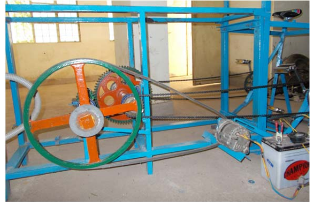
Fig. 3: Belt-pulley, alternator and storage system.
