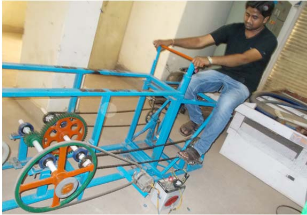
Fig. 2: Human paddle powered mechanical device for electricity generation.
